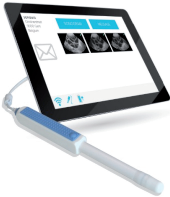
Fig. 1. — The Sonaura system consists of a dedicated tablet connected to a vaginal probe using USB technology.
